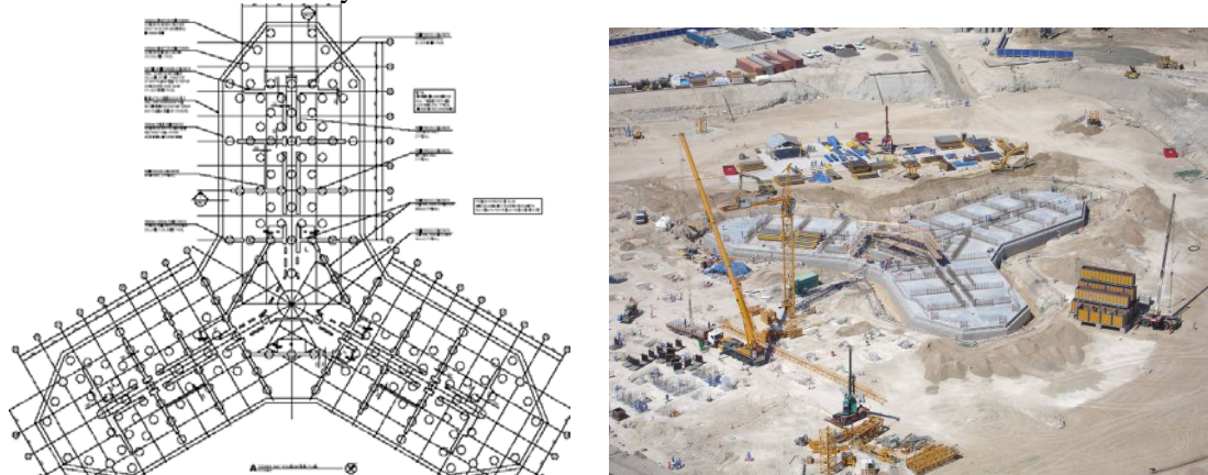
Figure 6. Tower raft foundation plan and photo of raft construction
